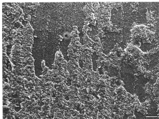
Figure 3 Scanning electron micrograph of an adhesive fracture surface of fracture type 2 (ceramic bracket, thermodebonding) with attached covering of coherent enamel particles. Bar = 50 \mu\text{m} .
